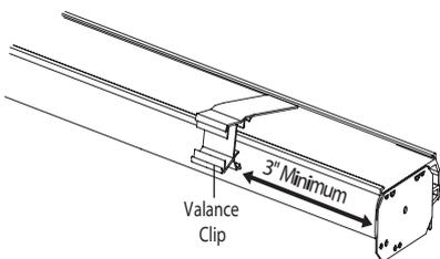
Note: Do NOT snap the valance clips completely onto the front of the headrail.
