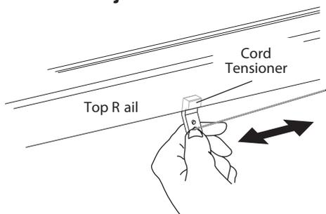
Install cord in tensioner. Slide cord tensioner to approximately 12" from the end of the headrail.
