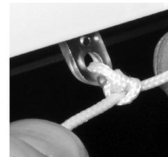
Move the moving rail to check the amount of tension on the shade. The moving rail should slide easily but there should be enough cord tension to hold the shade in place at any position.
