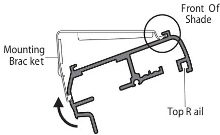
Slip the headrail into the installation brackets so that the front of the bracket slides under the front groove on the top of the rail. Gently roll the back of the headrail up and push back to snap into place.
